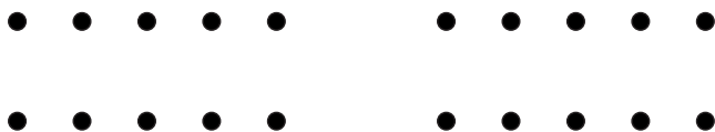
FIG. 6. A portion of a lattice consisting of linear clusters of five sites. An adsorbed molecule must lie entirely on a single cluster.
